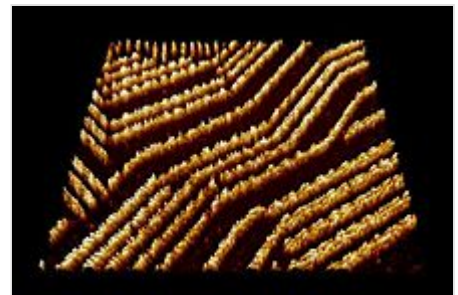
STM image of self-assembled supramolecular chains of the organic semiconductor quinacridone on graphite .
