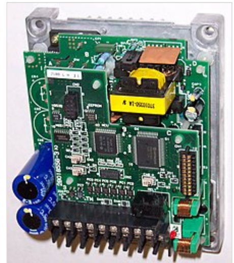
Hitachi J100 adjustable frequency drive chassis
